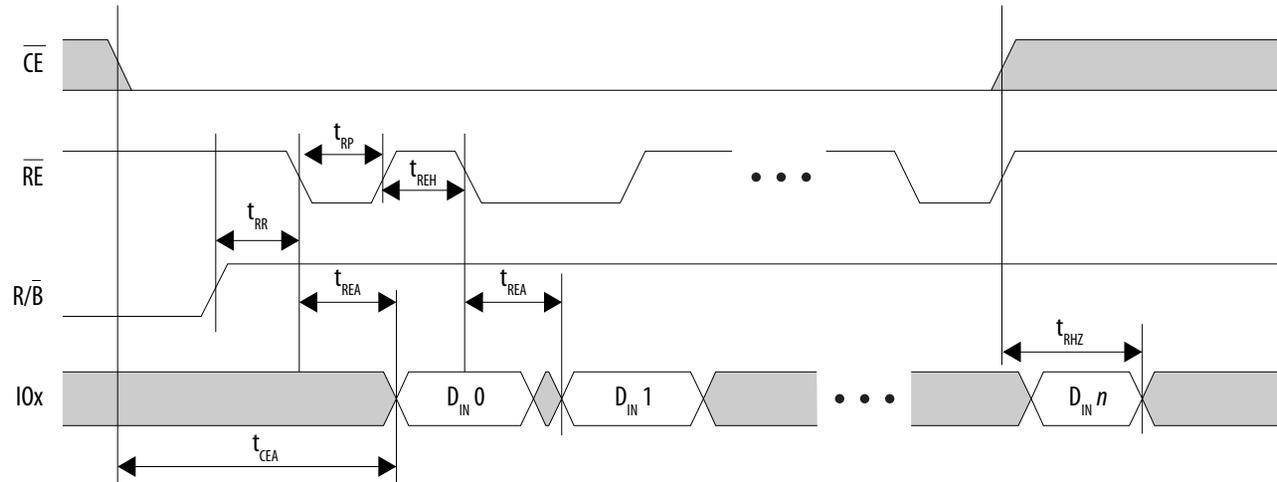
Figure 22. NAND Read Status Timing Diagram
