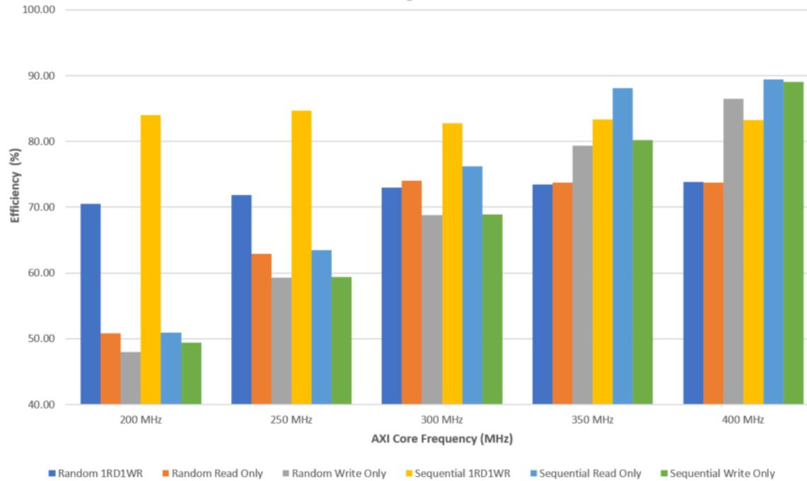
*Note:* These graphs show the Efficiency information for the HBM2 interface running at 800 MHz in an Intel Stratix 10 MX, NX, and DX 2100 device with -2 Speed Grade using 64B access, with the re-order buffer turned off and different AXI Transaction IDs enabled.
