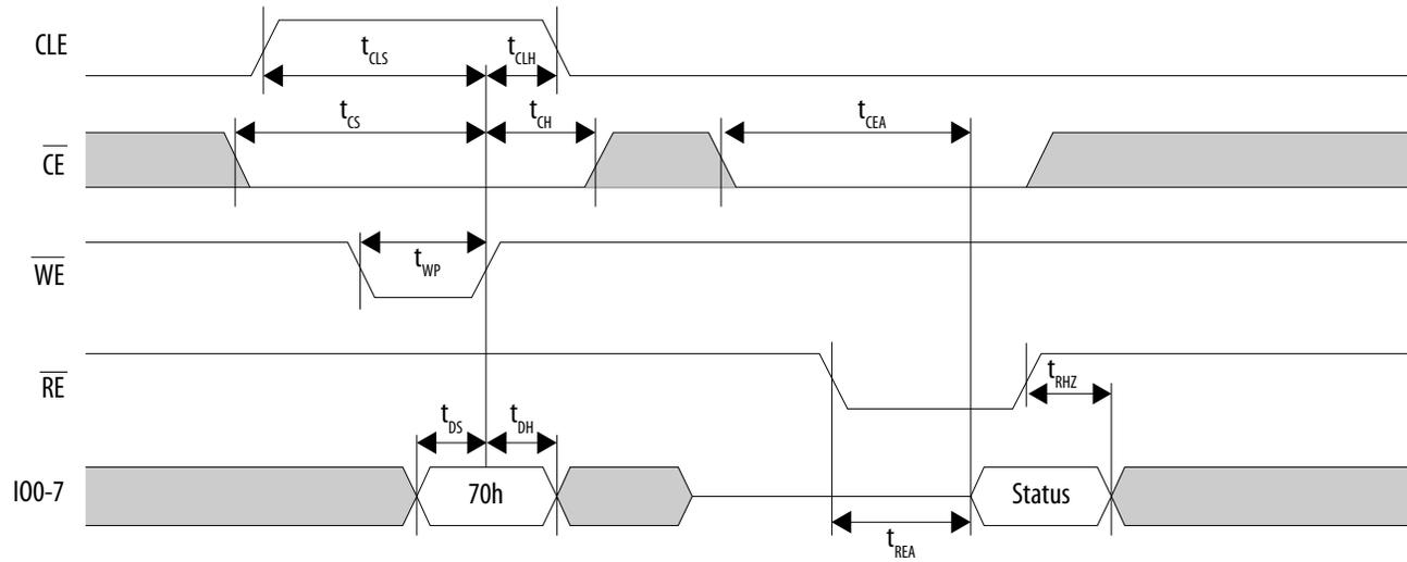
Figure 23. NAND Read Status Enhanced Timing Diagram
