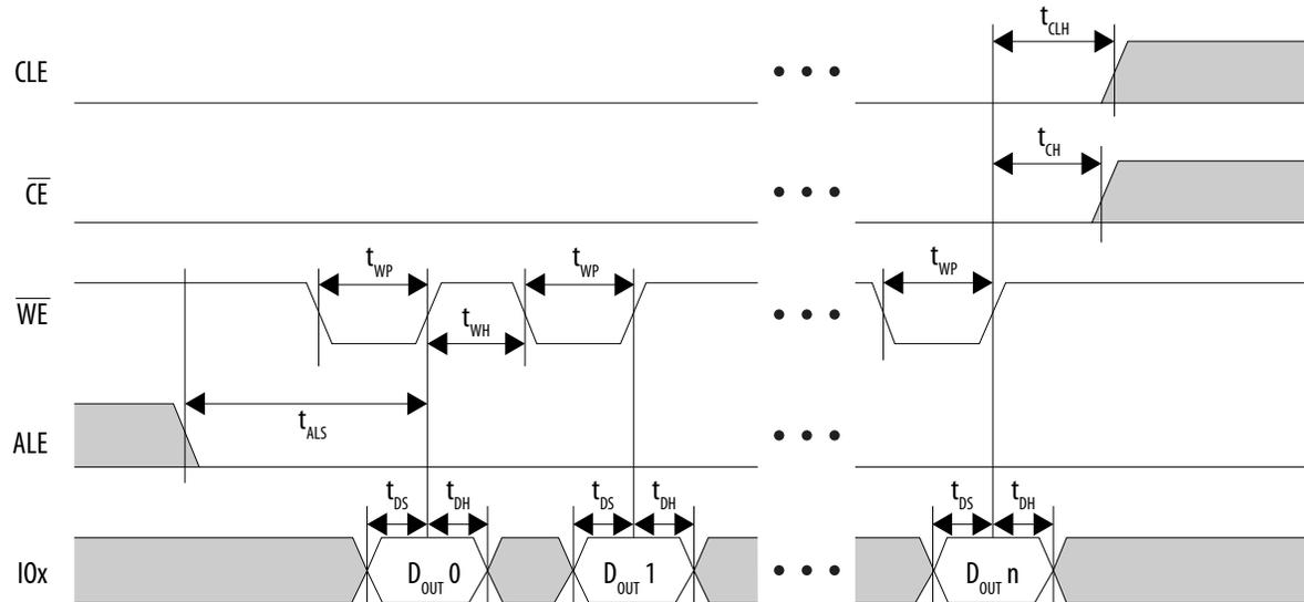
Figure 20. NAND Data Input Cycle Timing Diagram
