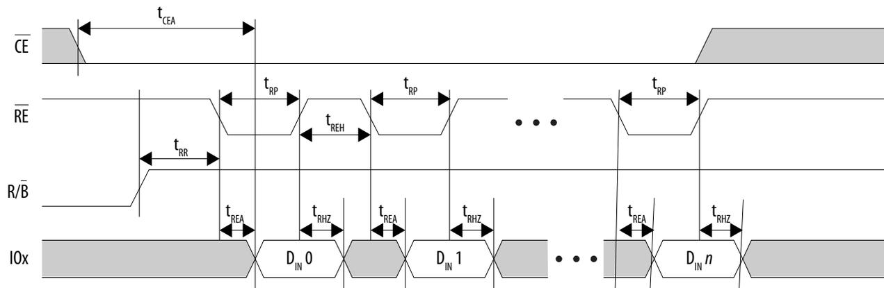
Figure 21. NAND Data Input Timing Diagram for Extended Data Output (EDO) Cycle
