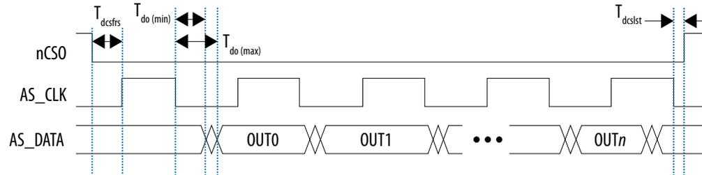
Figure 28. AS Configuration Serial Input Timing Diagram
