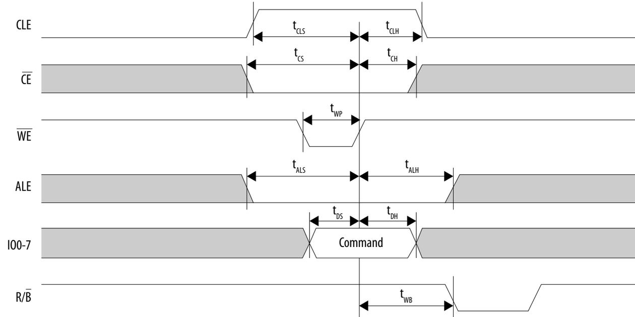
Figure 18. NAND Address Latch Timing Diagram
