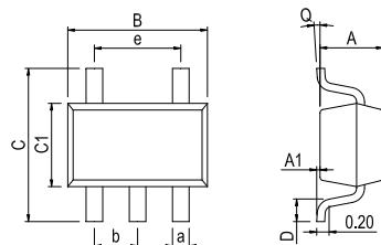
Dimensions In Millimeters(SOT-23-5)
