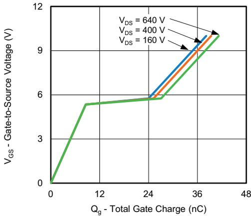
Fig. 7 - Typical Gate Charge vs. Gate-to-Source Voltage
