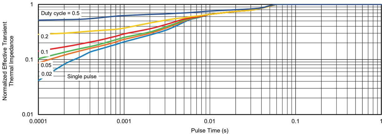
Fig. 12 - Normalized Transient Thermal Impedance, Junction-to-Case
