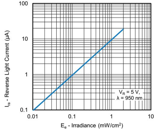
Fig. 3 - Reverse Light Current vs. Irradiance
