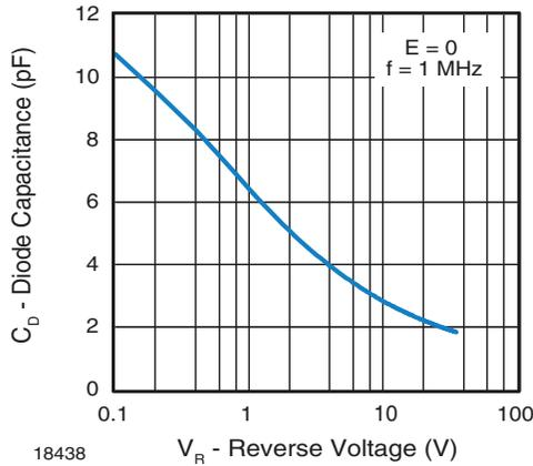
Fig. 5 - Diode Capacitance vs. Reverse Voltage
