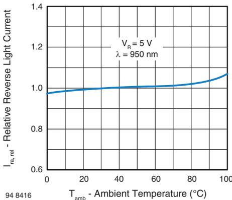
Fig. 2 - Relative Reverse Light Current vs. Ambient Temperature
