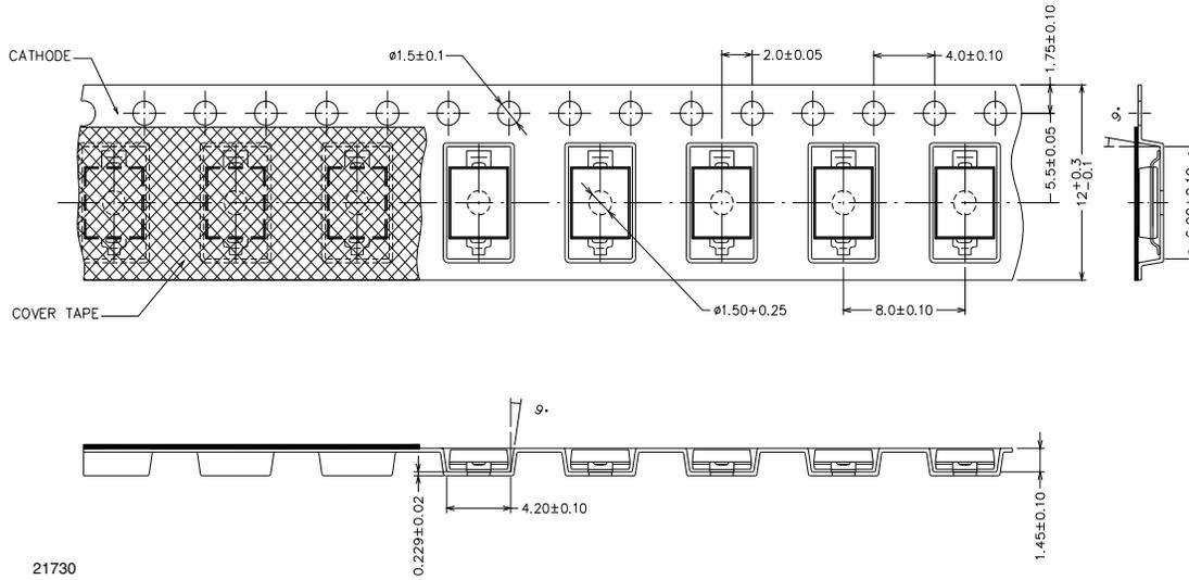
TAPING DIMENSIONS FOR VBP104SR in millimeters
