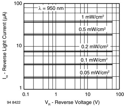
Fig. 4 - Reverse Light Current vs. Reverse Voltage
