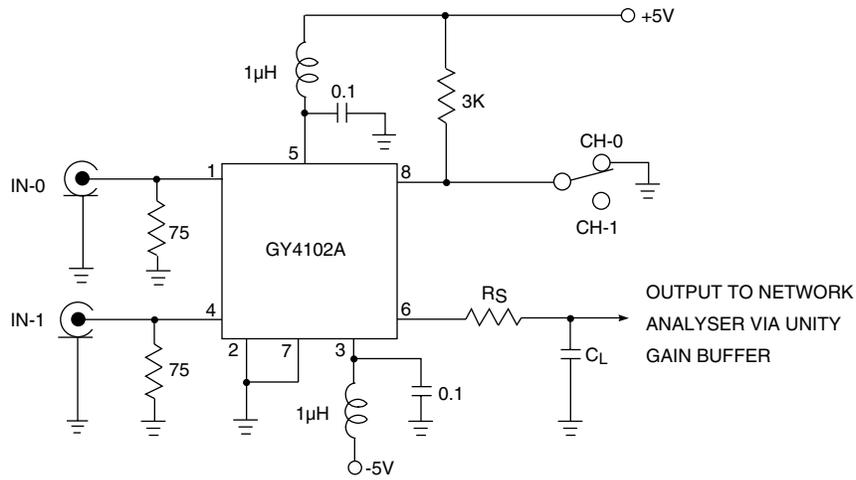
All resistors in ohms, all capacitors in microfarads unless otherwise stated
