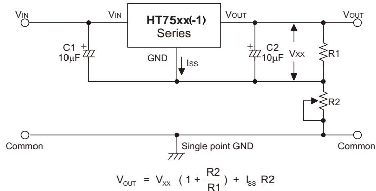
**Circuit for Increasing Output Voltage**
