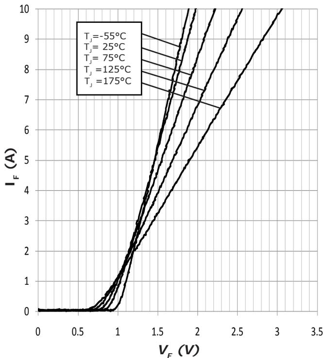
Figure 1. Forward Characteristics
