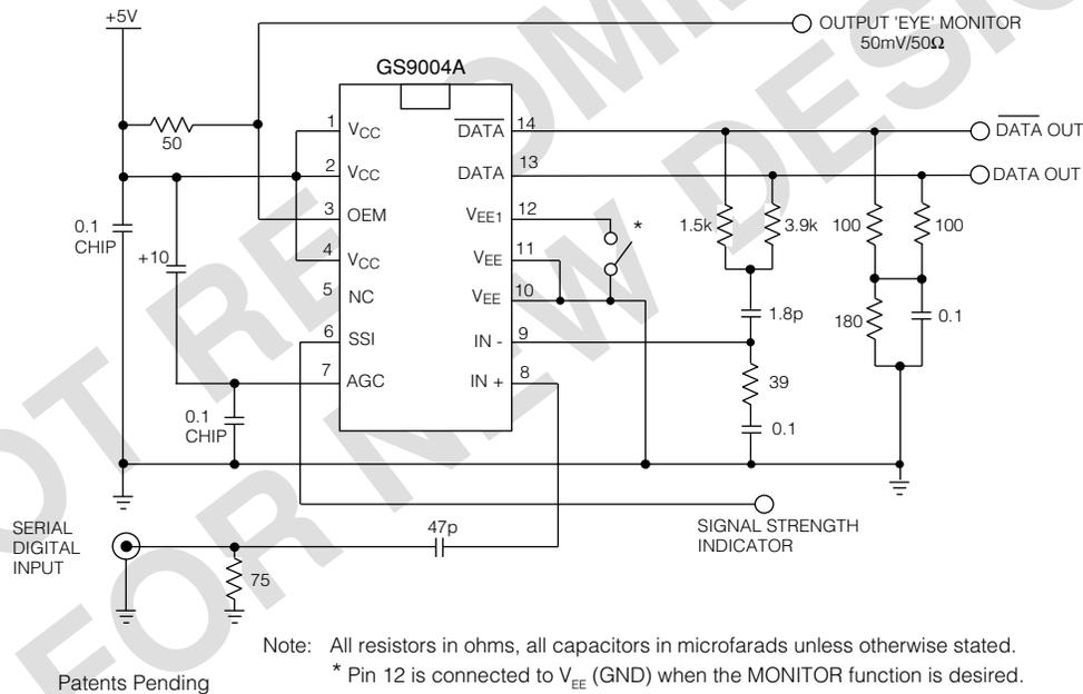
Fig. 1 Test Circuit
