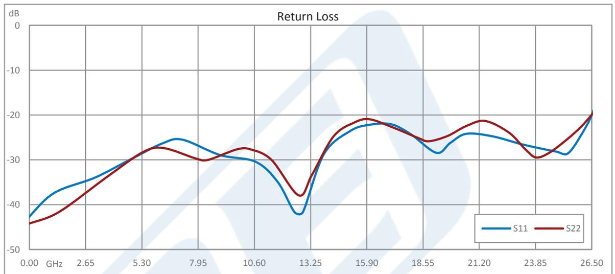
SMA Male to SMA Female Radius Right Angle Adapter, Functional Up to 26.5 GHz from Pasternack Enterprises has same day shipment for domestic and International orders. Our RF, microwave and millimeter wave products maintain a 99.4% availability and are part of the broadest selection in the industry.
