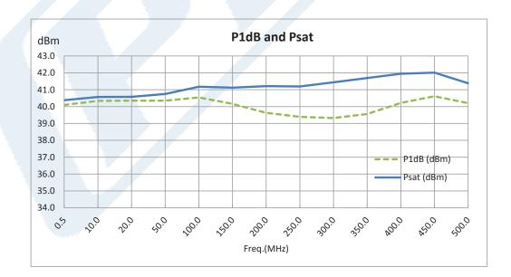
Click the following link (or enter part number in "SEARCH" on website) to obtain additional part information including price, inventory and certifications: 44 dB Gain, 8 Watt Psat, 0.5 MHz to 500 MHz, High Power LDMOS Amplifier, SMA Input, SMA Output, 42 dBm IP3, Class A/AB, with Heatsink PE15A5029F
