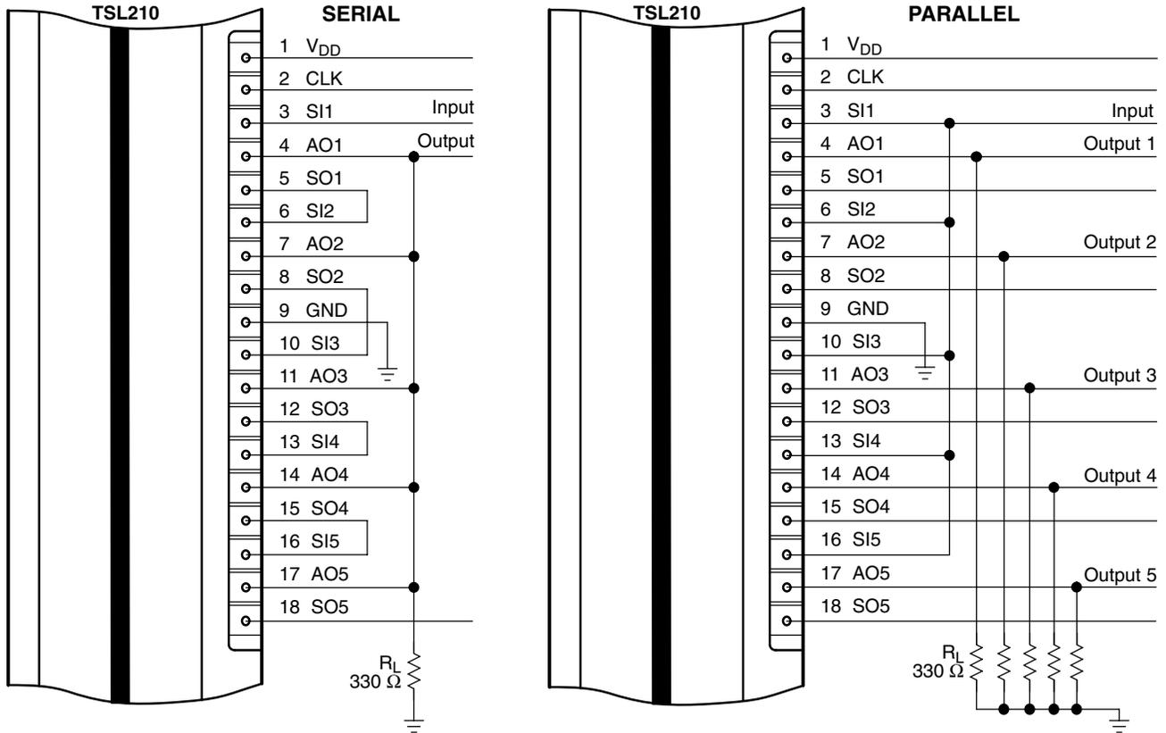
Figure 4. Connection Diagrams
