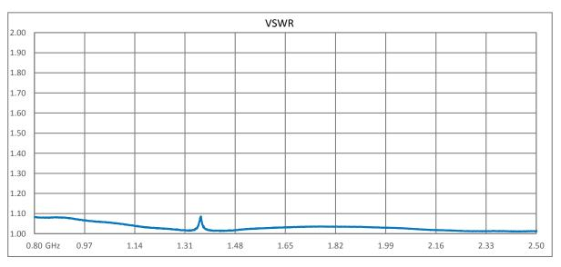
Click the following link (or enter part number in "SEARCH" on website) to obtain additional part information including price, inventory and certifications: TNC F/F Coaxial RF Surge Protector, 800MHz - 2.5GHz, 300W, IP67, 6 V Max., 175uJ, 20kA, Hybrid, Bracket Down, Hole Mount DGXZ+06TFTF-A
