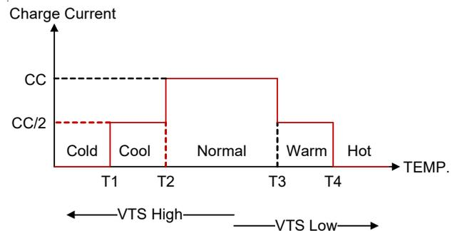
Thermal of battery can be monitored by TS PIN. There are 4 sections should be implemented in JEITA function. Base on  $R_{hot}$  and  $R_{cold}$ , RT1 and RT2 can be determined by equation (1) and equation (2).
