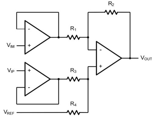
Figure 6. Instrument Amplifier
