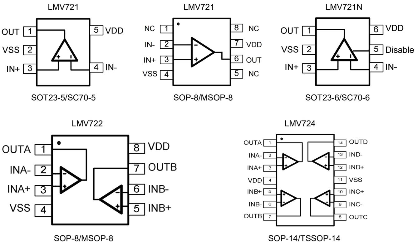
Figure 1. Pin Assignment Diagram
