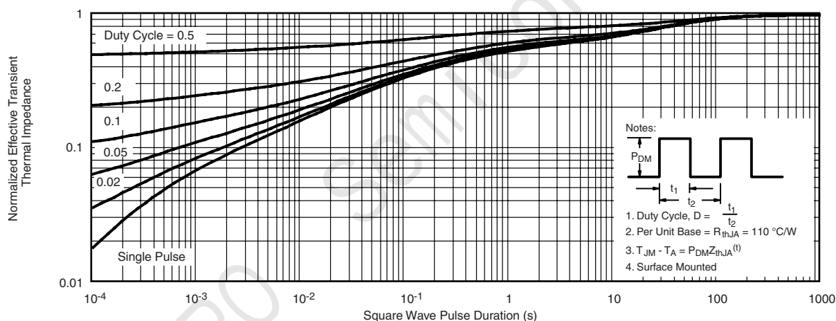
Normalized Thermal Transient Impedance, Junction-to-Ambient
