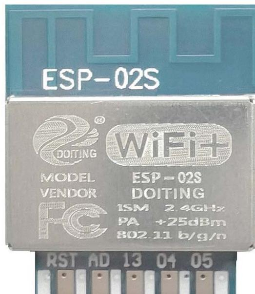
Fig.3.1 Shape for ESP-02S
