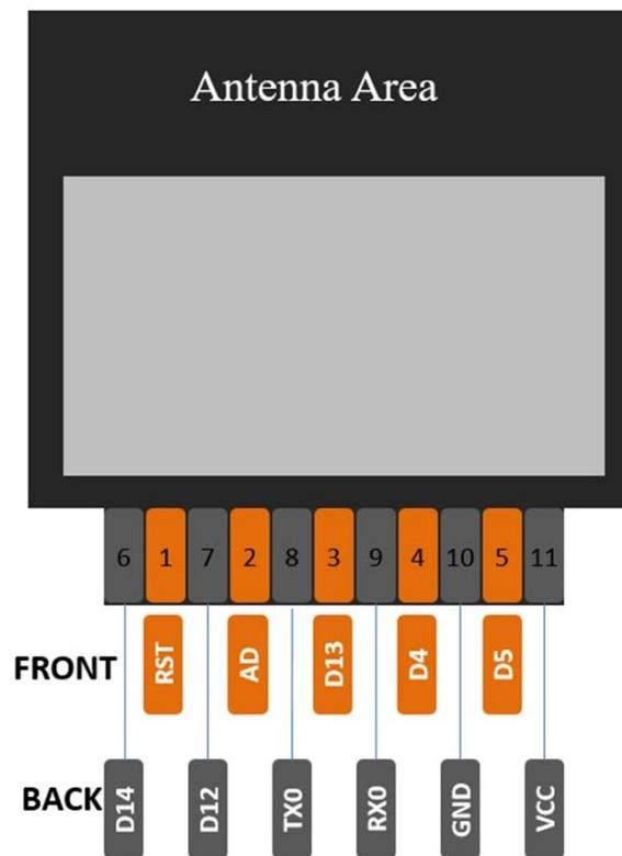
Fig. 2.1 ESP-02S Pins Definition
