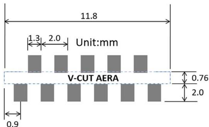
Fig. 3.3 PCB Layout for ESP-02S
