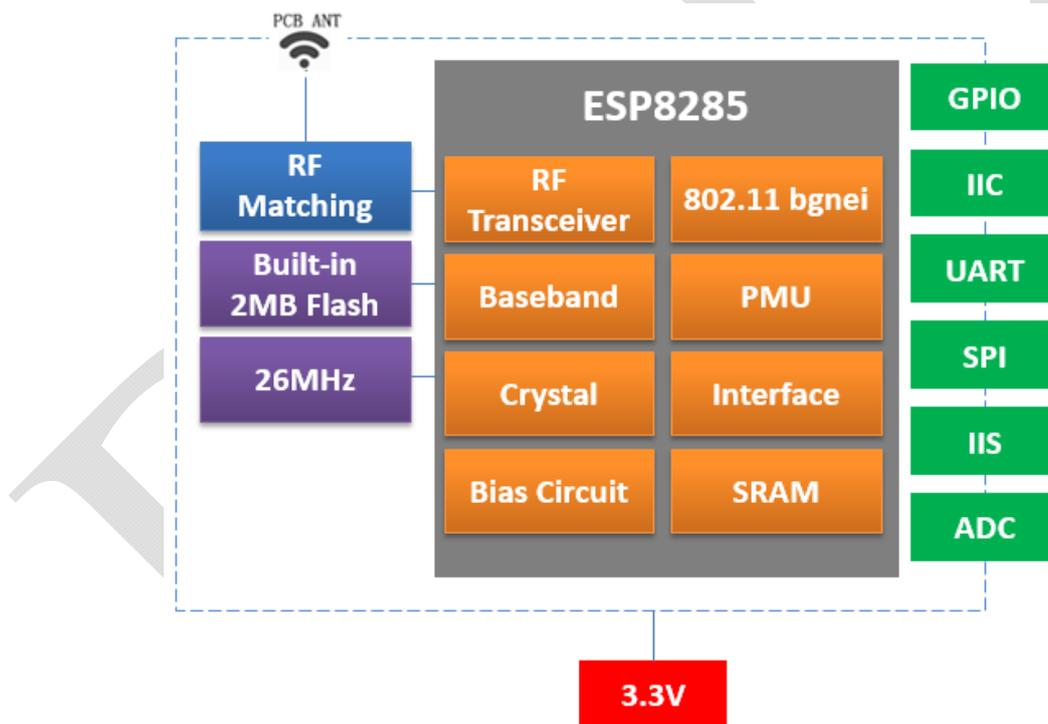
Fig. 1.1 ESP-02S Module Structure
