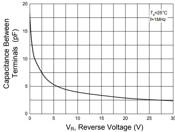
Figure 3. Capacitance Characteristics
