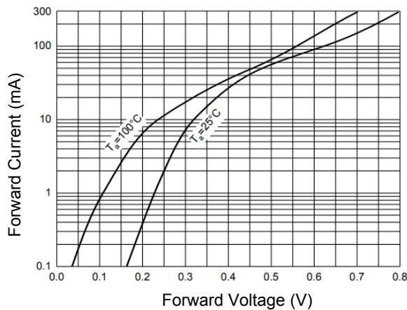
Figure 1. Forward Characteristics
