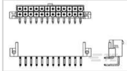
Rectangular Power Connector Type: **Header**Connector & Housing Type: **Plug**Connector System: **Wire-to-Board**Number of Positions: **12**Centerline (Pitch): **4.2 mm [.165 in]**
