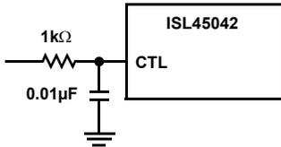
**FIGURE 3. EXTERNAL ESD PROTECTION ON CTL PIN**
