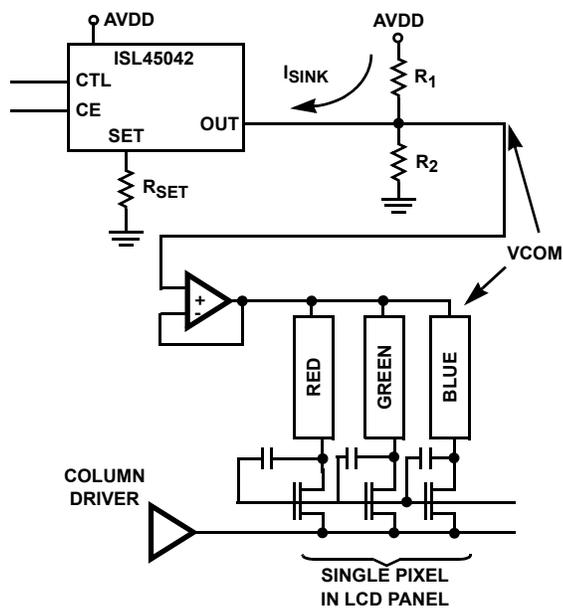
FIGURE 1. VCOM ADJUSTMENT IN AN LCD PANEL
