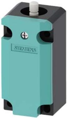
Position switch basic switch plastic 40 mm, according to EN 50041 Increased corrosion protection Device connection 1 x (M20 x 1.5) 1 NO/2 NC quick action contacts functional at -40 °C Shock and vibration test according to EN 61373, Category 1B
