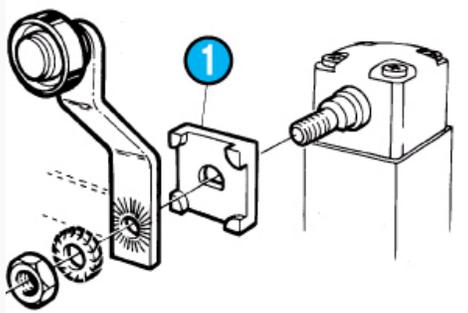
Lever settings or positions dictated by direction in which block 1 is fitted
