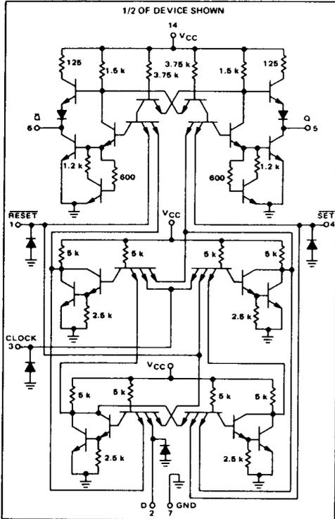
This dual type D flip flop triggers on the positive edge of the clock input. During the clock transition the state of the D input is transferred to the Q output. The device is useful in shift registers and simple counters.
