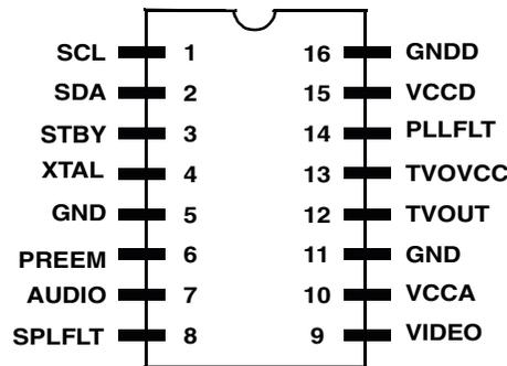
Figure 1. Pin Connection Diagram
