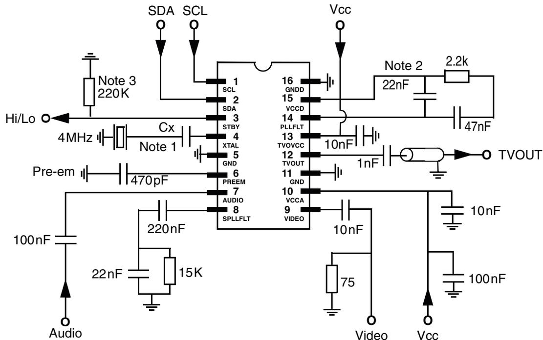
Note 1:  $C_x$  value depends on crystal characteristics;  $C_x = 27\text{pF}$  on Motorola application board.
