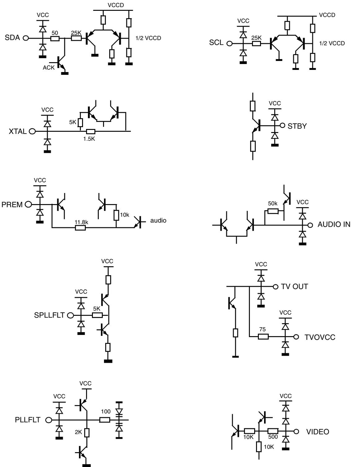
Figure 6. Pin Schematics
