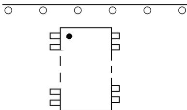
Component Orientation: Arrange parts with the pin 1 side closest to the tape's round sprocket holes on the tape's trailing edge.
