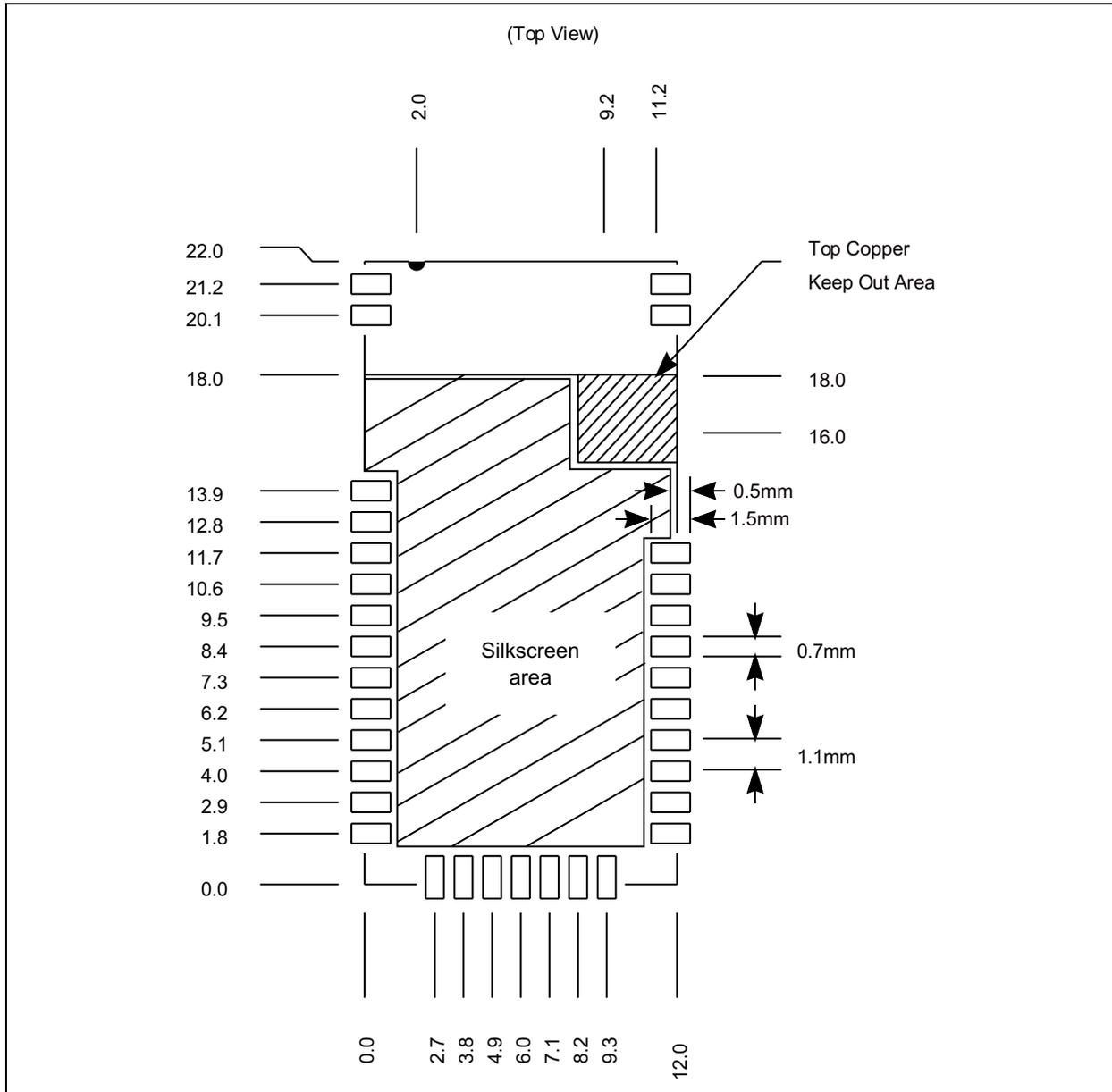
The following figure illustrates the recommendations for mounting the RN4678 on the host PCB, and also shows the minimum ground plane area to the left and right of the module for the best antenna performance.
