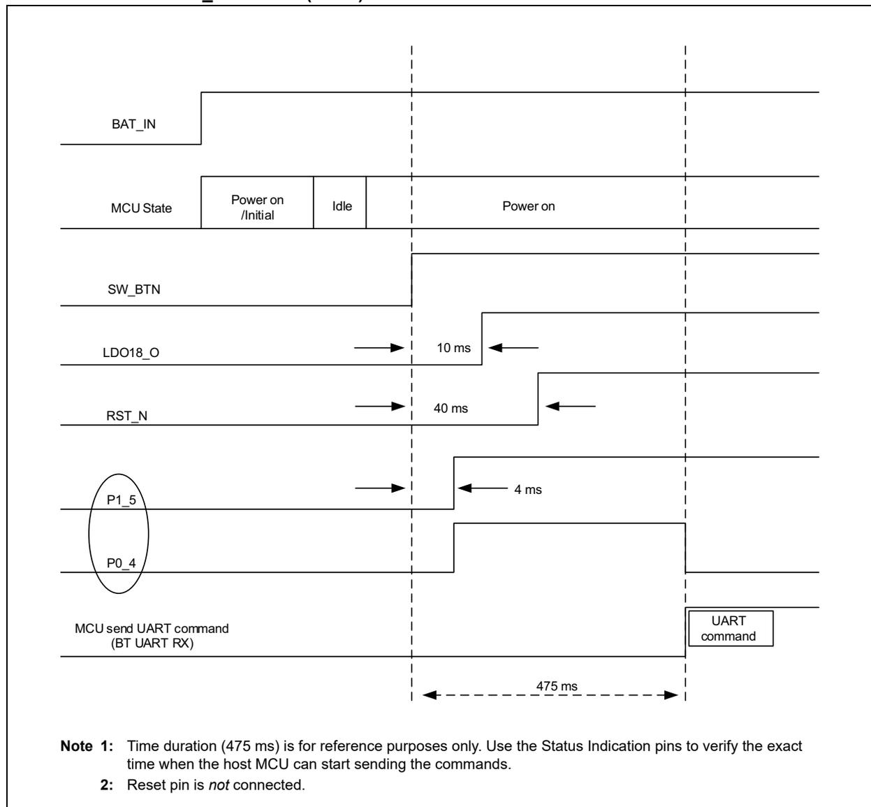
**FIGURE 2-3: SW\_BTN TIME (LOW) AT ACCESS STATES<sup>(1)</sup>**
