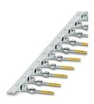
Crimp contact, Pin, rolled, Taped product, number of pieces per reel: 500, contact diameter: 1 mm, crimp range:  $0.22~\text{mm}^2$ ...  $0.56~\text{mm}^2$ , Item is lead-free in accordance with RoHS II without Exemption 6c (Pb <0.1%)
