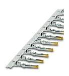
Crimp contact, Socket, rolled, Taped product, number of pieces per reel: 500, contact diameter: 1 mm, crimp range: 0.22 mm $^2$  ... 0.56 mm $^2$ , Item is lead-free in accordance with RoHS II without Exemption 6c (Pb <0.1%)
