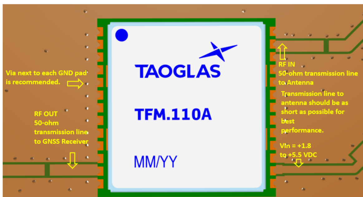
TFM.110A module mounted on a PCB, showing transmission lines and integration notes.
