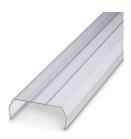
Cover profile, for covering terminal strips, snapped onto APT-ME cover profile carrier or APH-ME end bracket. A cover profile carrier should be positioned at the ends and at intervals of around 40 cm. Length supplied: 1 m
