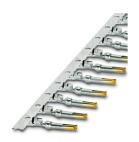
Crimp contact, Socket, rolled, Taped product, number of pieces per reel: 500, contact diameter: 1 mm, crimp range: 0.08  $\rm mm^2$  ... 0.22  $\rm mm^2$
