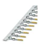
Crimp contact, Pin, rolled, Taped product, number of pieces per reel: 10000, contact diameter: 1 mm, crimp range: 0.22 mm $^2$  ... 0.56 mm $^2$ , Item is lead-free in accordance with RoHS II without Exemption 6c (Pb <0.1%)
