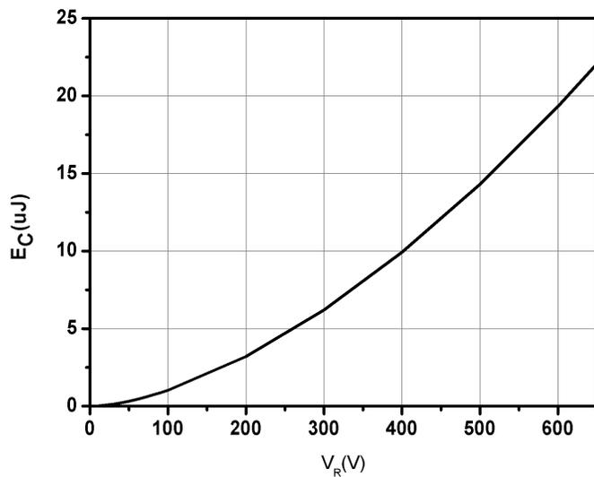
Fig.5-Capacitance Stored Energy
