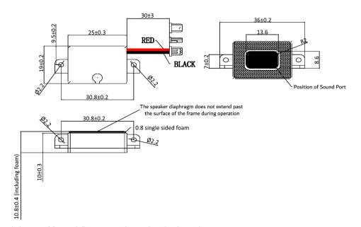
General tolerance =  $\pm 0.3$  mm and all measurements in mm unless otherwise noted
