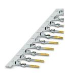
Crimp contact, Pin, rolled, Taped product, number of pieces per reel: 500, contact diameter: 1 mm, crimp range:  $0.08~\text{mm}^2$  ...  $0.22~\text{mm}^2$
