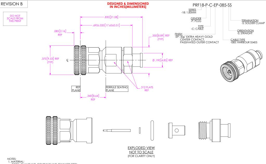
BODY, CLAMP NUT, COUPLING NUT: STAINLESS STEEL.
