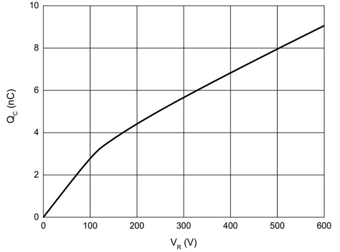
Fig. 5 - Capacitance Stored Energy
