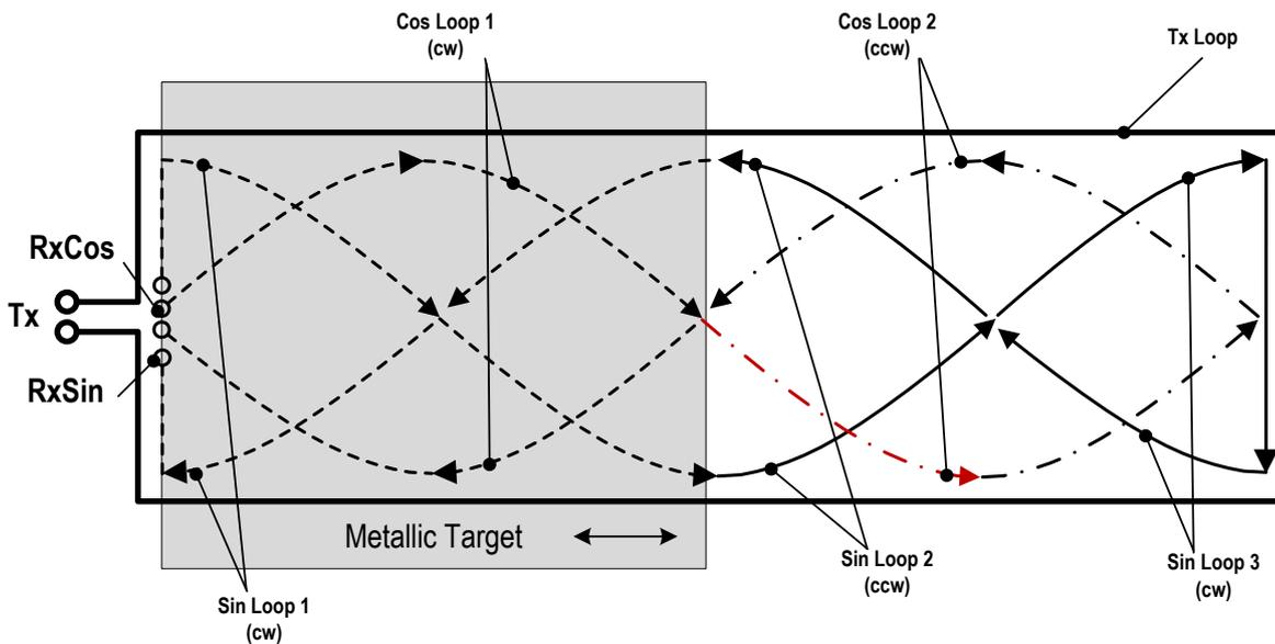
Figure 3. Coil Design for a Linear Motion Sensor
