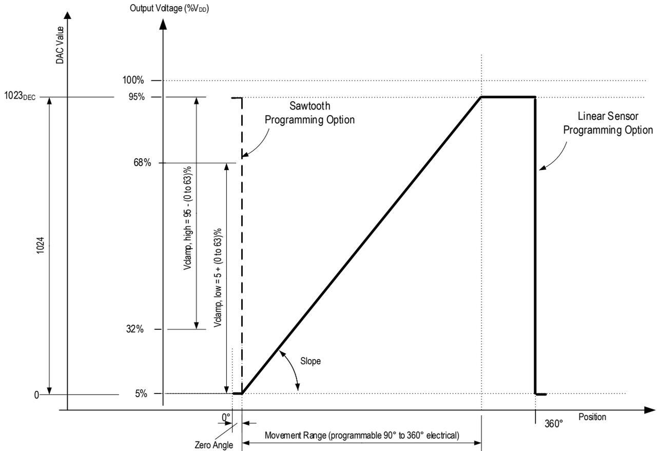
Note: An example of 5% and 95% clamping levels and a rising slope setting is illustrated.
