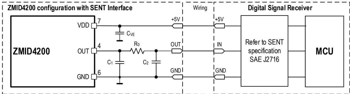
Figure 12. External Components for ZMID4200 SENT Interface
