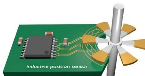
Figure 23. Example Setup: Side-Shaft Rotation, 6 x 60°
