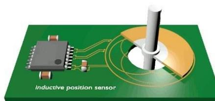
Figure 22. Example Setup: Through-Shaft Rotation, 1 x 360°
