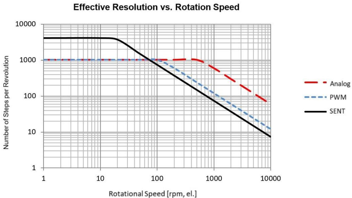
Figure 17. Relationship between Resolution and Rotational Speed
