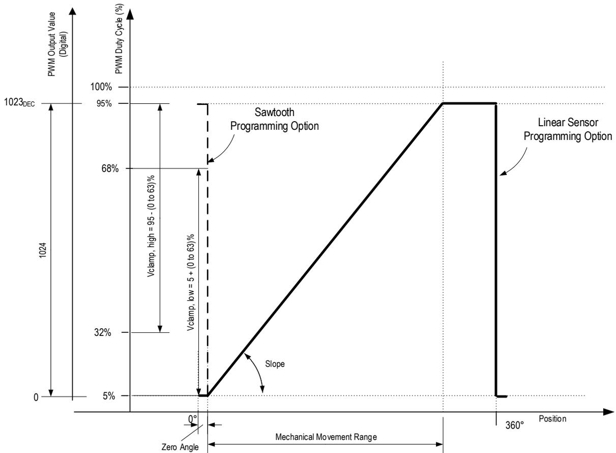
Note: An example of 5% and 95% clamping levels and a rising slope setting is illustrated.
