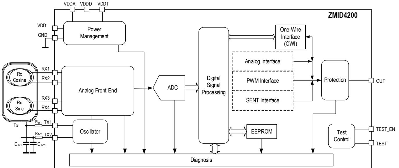
Figure 4. Block Diagram
