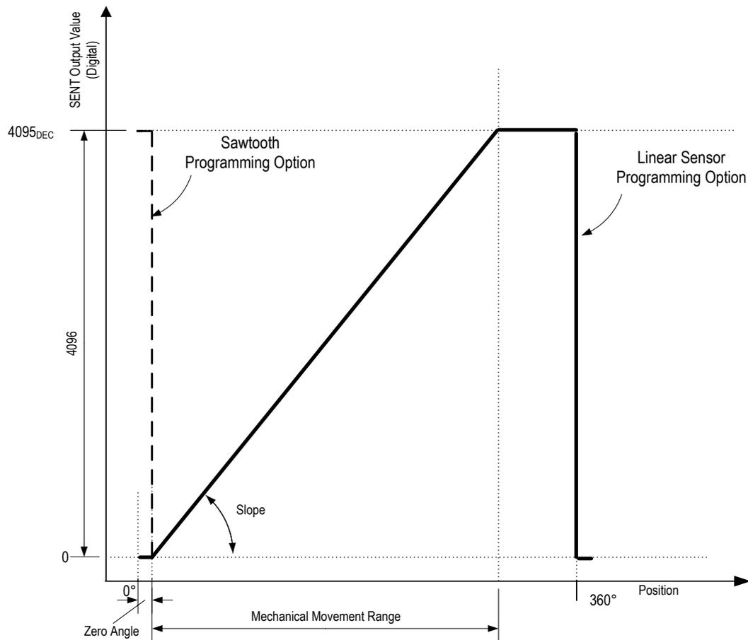
Note: An example using the rising slope setting is illustrated.
