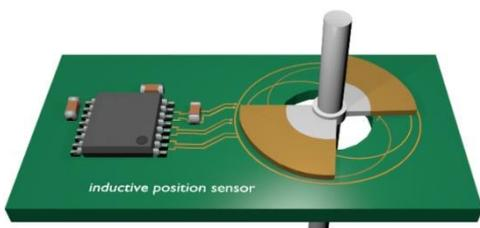
Figure 21. Example Setup: Through-Shaft Rotation, 2 x 180°
