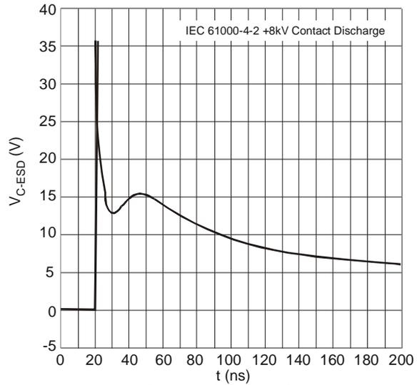
Figure 8 Typical Clamping Performance @ 8kV Contact Discharge
