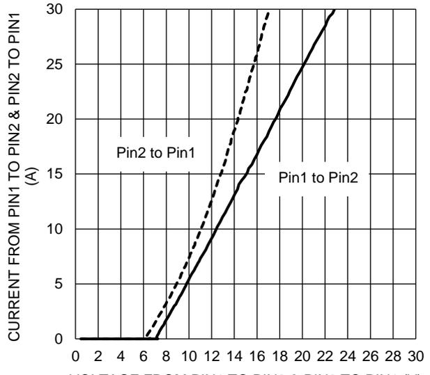
Figure 10 TLP Curve ( $t_p = 100\text{ns}$ )
