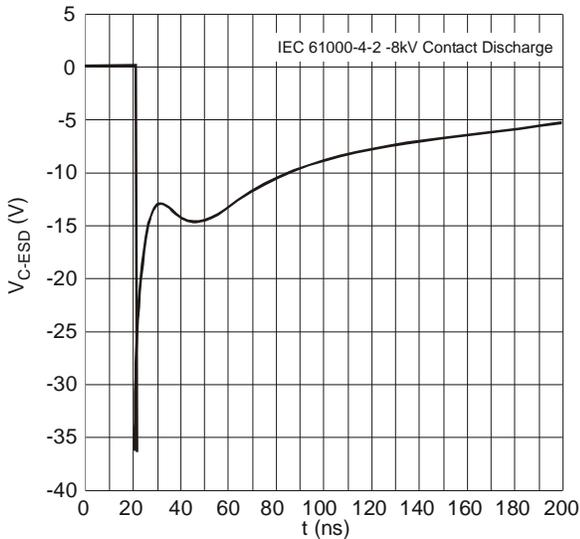
Figure 9 Typical Clamping Performance @ -8kV Contact Discharge
