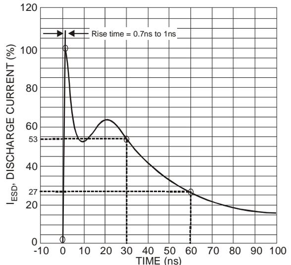
Figure 6 ESD Discharge Current Wave Form IEC 61000-4-2 (330Ω/150pF)
