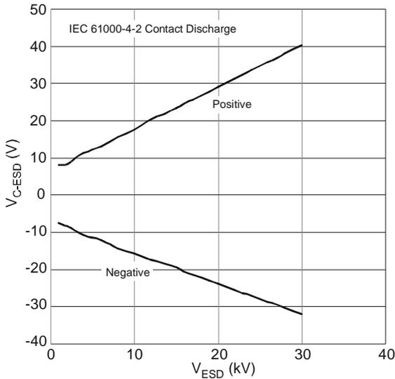
Figure 7 Typical Clamping Voltage vs. Contact Discharge Voltage
