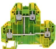
Protective-earth double-level terminal, Screw connection, Mounting type: Mounting rail TS 35/7.5, Rated cross-section: 4 mm<sup>2</sup>, Width: 6.1 mm, Colour: Green-yellow
