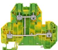
Protective-earth double-level terminal, Screw connection, Mounting type: Mounting rail TS 35/7.5, Rated cross-section: 2.5 mm<sup>2</sup>, Width: 5.1 mm, Colour: Green-yellow
