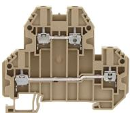
Double-level terminal, Screw connection, Mounting type: Mounting rail TS 35/7.5, Rated cross-section: 2.5 mm<sup>2</sup>, Width: 5.1 mm, Colour: Beige
