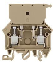
Fuse-disconnect terminal, Screw connection, Mounting type:Mounting rail TS 35/7.5 and TS 32, Rated cross-section: 10 mm<sup>2</sup>, Width: 8 mm, Colour: Beige
