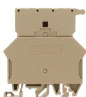
Fused terminal with disconnect plug, Screw connection, Mounting type:Mounting rail TS 35/7.5 and TS 32, Rated cross-section: 10 mm<sup>2</sup>, Width: 10 mm, Colour: Beige
