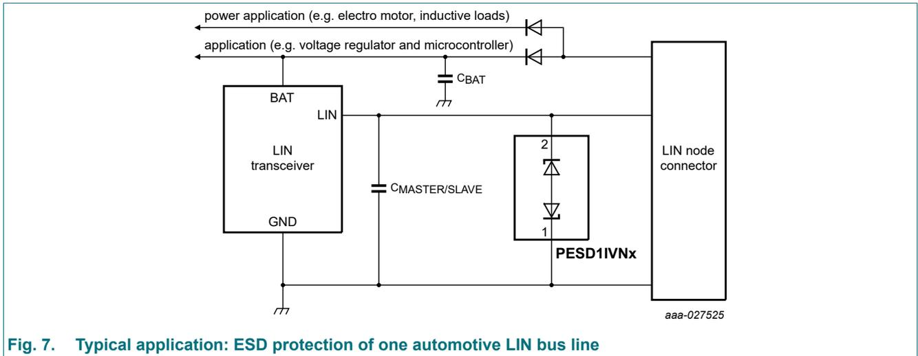
Fig. 7. Typical application: ESD protection of one automotive LIN bus line
