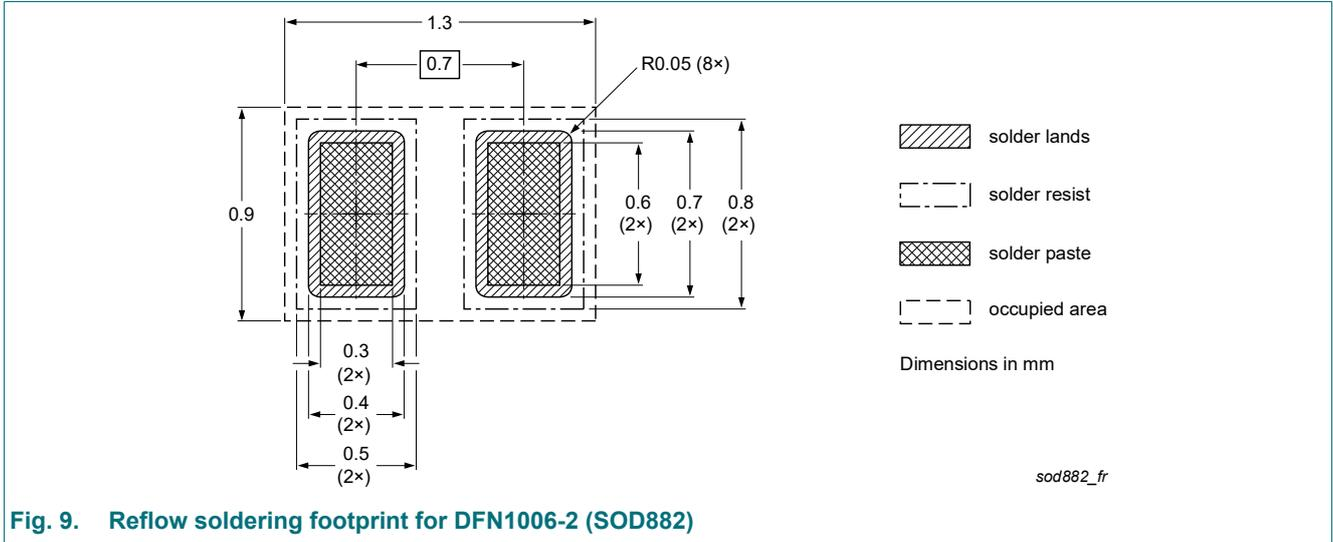
Fig. 9. Reflow soldering footprint for DFN1006-2 (SOD882)
