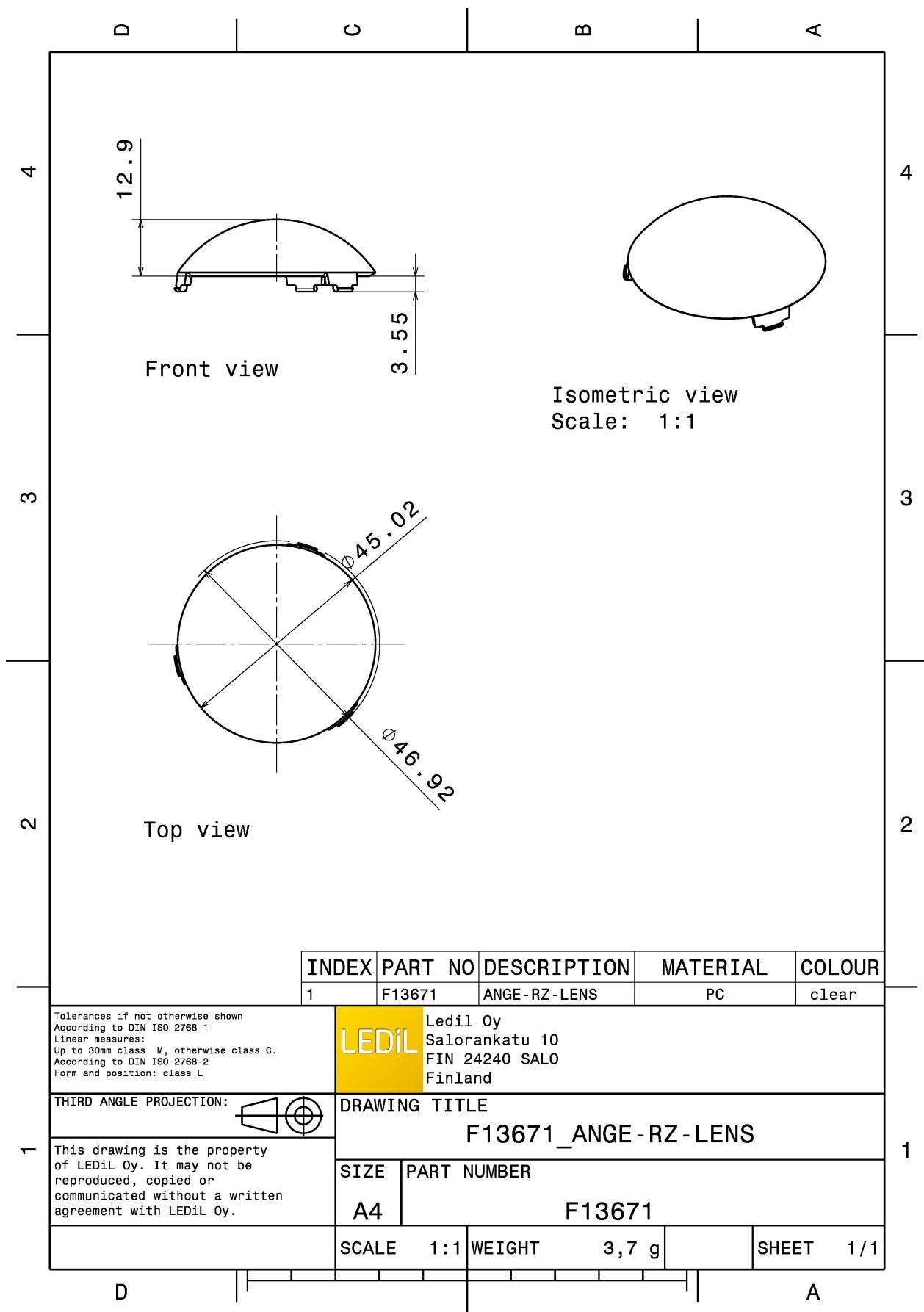
See also our general installation guide: [www.ledil.com/installation\\_guide](http://www.ledil.com/installation_guide)
