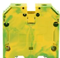
Protective earth terminal, Screw connection, Mounting type: Mounting rail TS 35/7.5, Rated cross-section: 50 mm<sup>2</sup>, Width: 18.5 mm, Colour: Green-yellow
