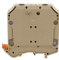
Feed-through terminal, Screw connection, Mounting type:Mounting rail TS 35/7.5 and TS 32, Rated cross-section: 50 mm<sup>2</sup>, Width: 20 mm, Colour: Beige
