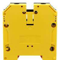
Feed-through terminal, Screw connection, Mounting type: Mounting rail TS 35/7.5, Rated cross-section: 70 mm<sup>2</sup>, Width: 20.5 mm, Colour: Black-yellow
