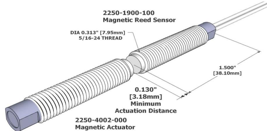
All measurements are in Inches [millimeters]
