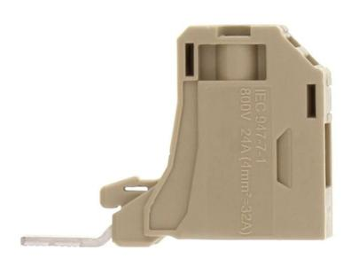
Measurement pick-off terminal, Screw connection, Mounting type: On base, Rated cross-section: 2.5 mm², Width: 5.9 mm, Colour: Beige
