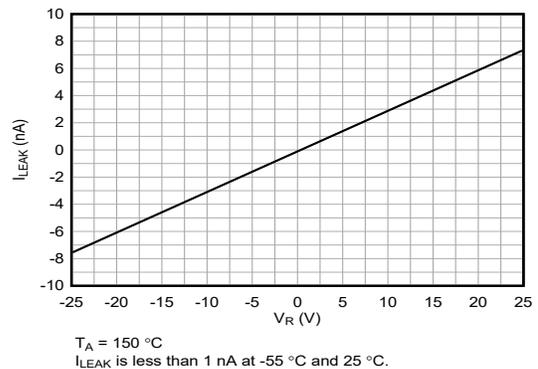
**Figure 6-6. Leakage Current vs. Bias Voltage Across Temperature**
