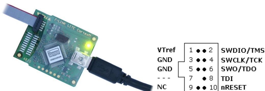
Figure 3 – SEGGER J-Link Lite Cortex-M 9-Pin JTAG with pinout (Rev 2.X+)
