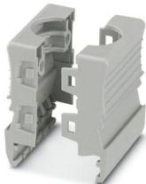
Cable housing, pitch: 31.2 mm, depth: 36.8 mm, width: 31.2 mm, height: 19.9 mm, number of positions: 6, color: gray
