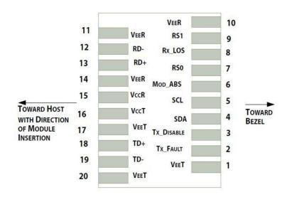
Pin-out of connector Block on Host board
