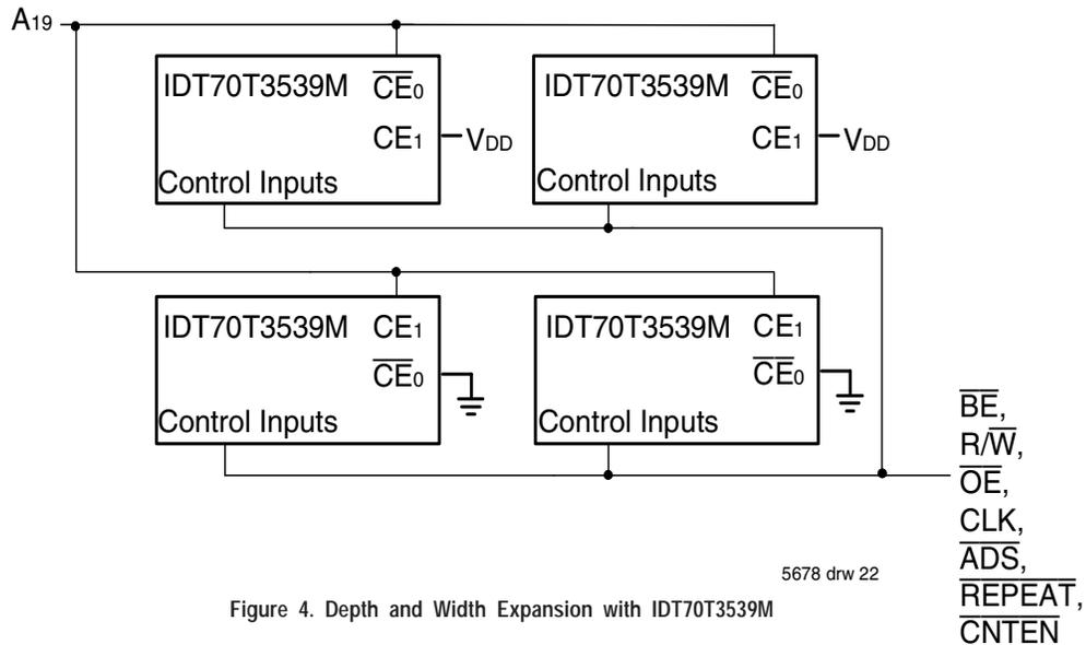
Figure 4. Depth and Width Expansion with IDT70T3539M
