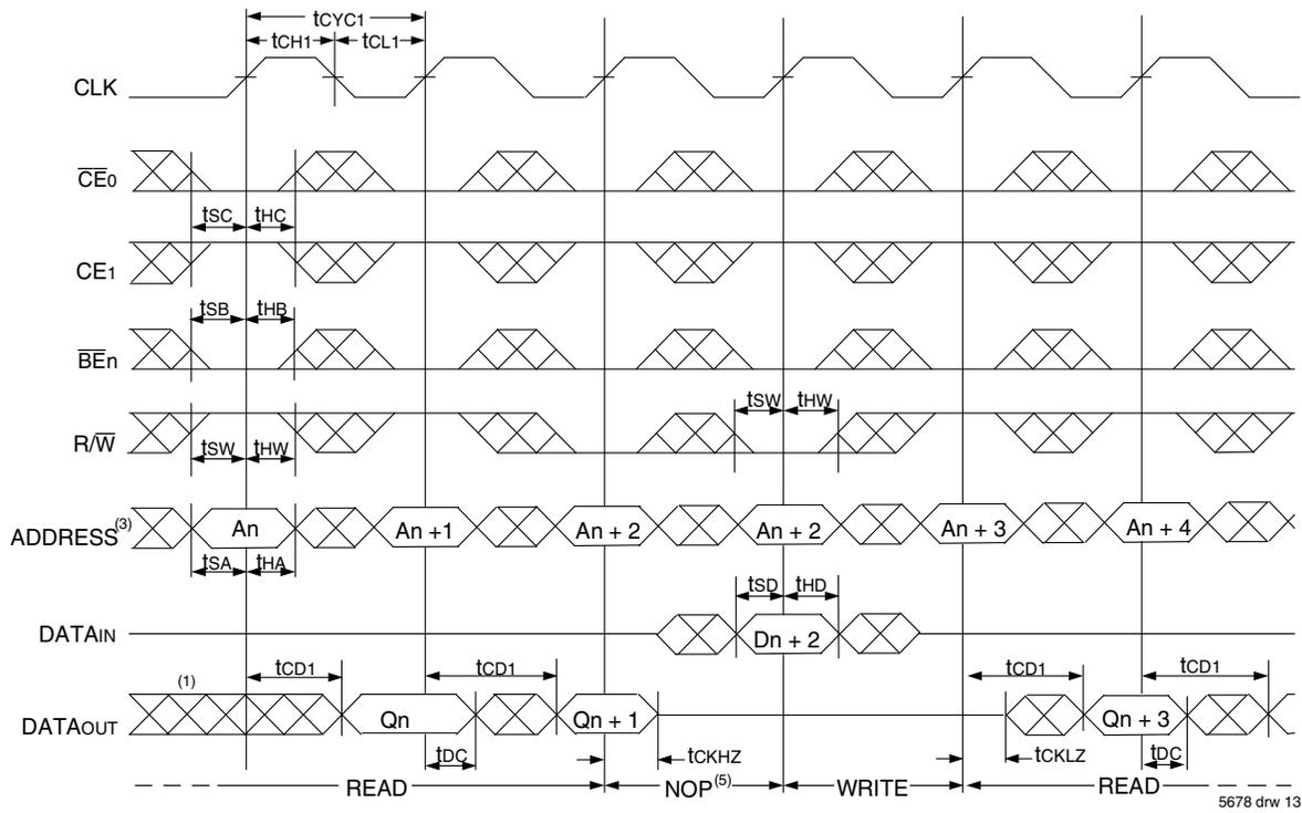
Timing Waveform of Flow-Through Read-to-Write-to-Read ( $\overline{OE}$  Controlled)<sup>(2)</sup>
